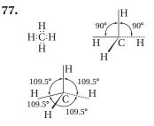
The first sketch is tetrahedral. The second sketch is a tetrahedron. The bond angles in the first sketch are not all the same; some are 90°. The bond angles in the second sketch are all 109.5° The second sketch is correct. (Note: The wedge-shaped lines come out of the page; the dotted lines recede into the page.)
